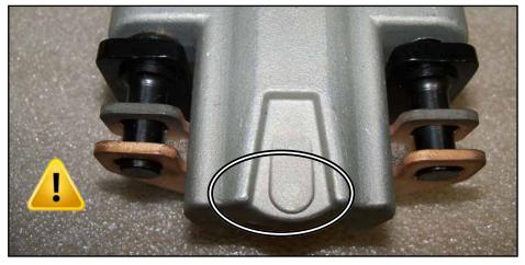
When installing Calipers ensure that Bleeders face UP.
