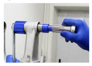
**g.** Assemble the bearing driver as shown in Fig 4. Tighten screw until the driver bottoms out on the inside bearing surface.
