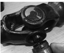
**5:** Repeat this procedure on the other side and remove the yoke from the U-Joint.
