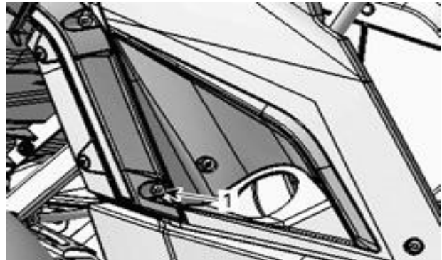
REAR RH SIDE - OUTSIDE VIEW. 1. M6 X 30 Torx screw.
