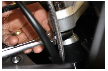
Remove the small nut and you will then be able to lower the fork tube on that side. Move the cables to the outside of the fork.
