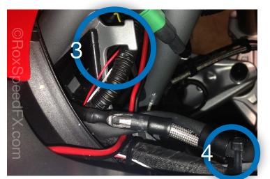
Remove the zip tie that is currently holding the brake side cables in AREA 3 and zip tie the cables to the tic-tac shaped hole in the frame in AREA 4. Hint: look for this shape: O. After rerouting the cables proceed with installing your Rox® Bar Risers. Always check to ensure your cables aren't under tension when fully turned in both directions!
