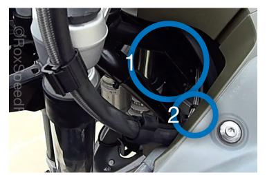
Remove the zip tie that is currently holding the clutch side cables in AREA 1 and then zip tie the cables to the tic-tac shaped hole in the frame in AREA 2. Hint: Look for this shape: O. Note: Your stock bike may or may NOT have a zip tie holding the cables currently.
