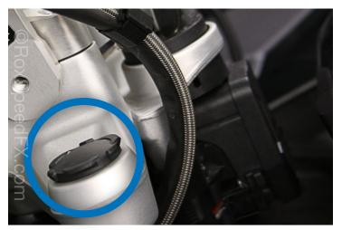
Place the motorcycle on its center stand. You will be working on one side of the bike from start to finish before beginning the other side. Look at the top of the triple clamp and remove any plastic that may be covering the top of the fork tubes (See photo). We use a flathead screwdriver and very carefully pry it up.
