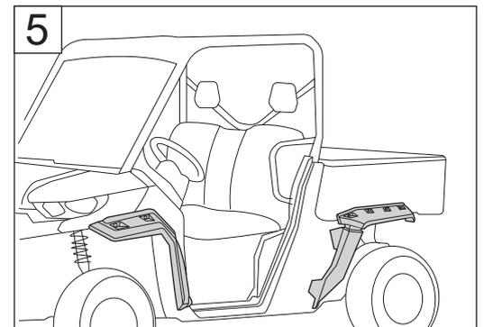
**STEP 4:** Install RH lower rear fender [6] to vehicle body panel.
