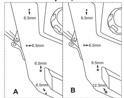
**STEP 1:** Place RH front fender [2] against vehicle body panel, mark and drill six 3mm holes. Secure the fender [2] with six self-tapping screws [7] and washers [12].
