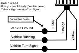
4. Test the function of the running light and turn signals before riding.
