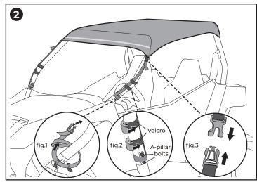
2 Unbuckle two front corner straps. Cinch the straps down between the two A-pillar bolts to keep them in place (fig.1). Attach the Velcro strips to roll bar (fig.2). Reinsert the buckle to the soft top (fig.3).
