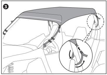
3 Unbuckle two rear corner straps. Route the buckle down around the seat belt mounting bracket and loop back up to the soft top.
