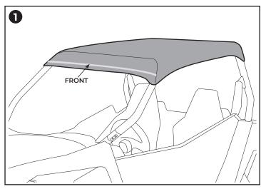
Place the soft top on the roof frame, with the "FRONT" tab toward the front of the vehicle.
