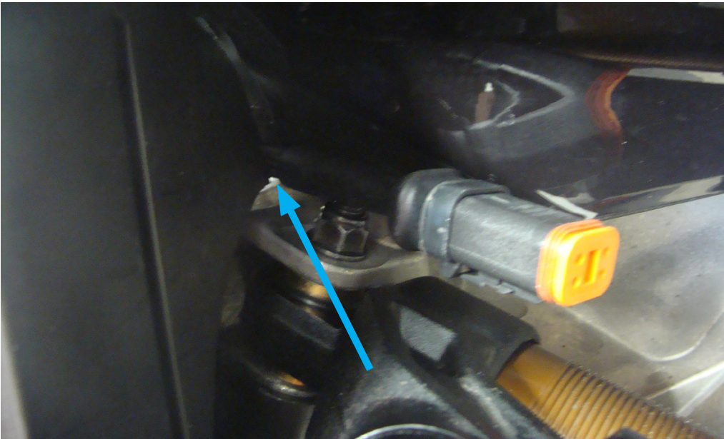
Figure 21: wiring after it is passed between the pans
