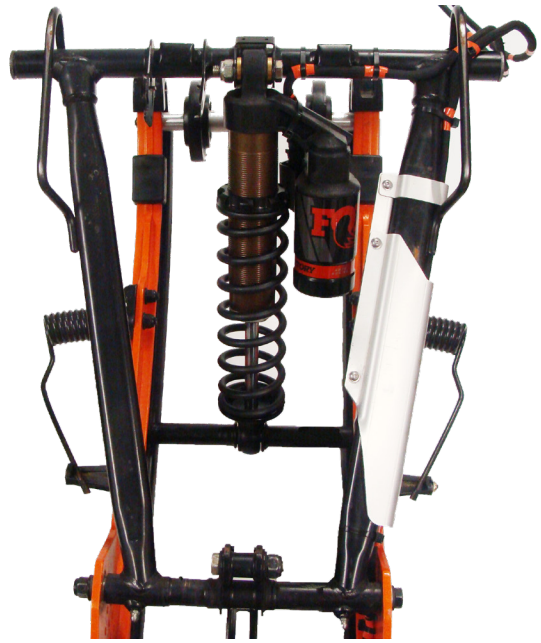
Figure 7: Orientation of front track shock reservoir
