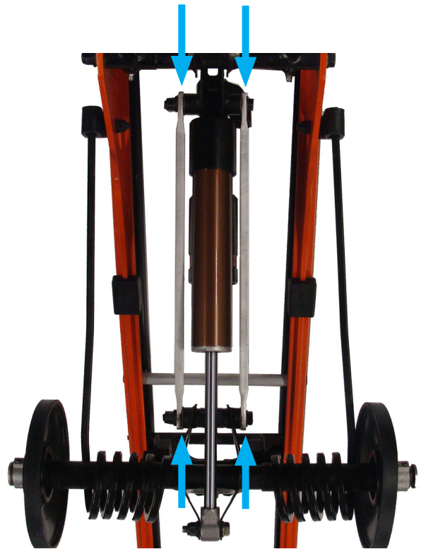
Figure 8: Orientation of rear track shock reservoir. Four arrows point to washer locations.
