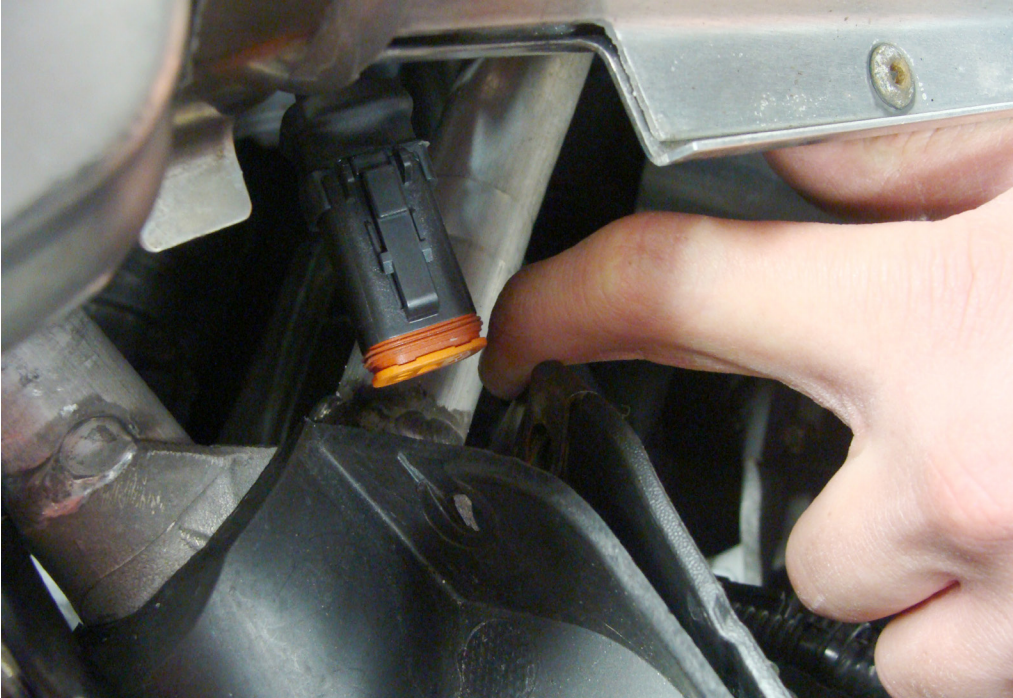
Figure 20: wiring before it is passed between the pans
