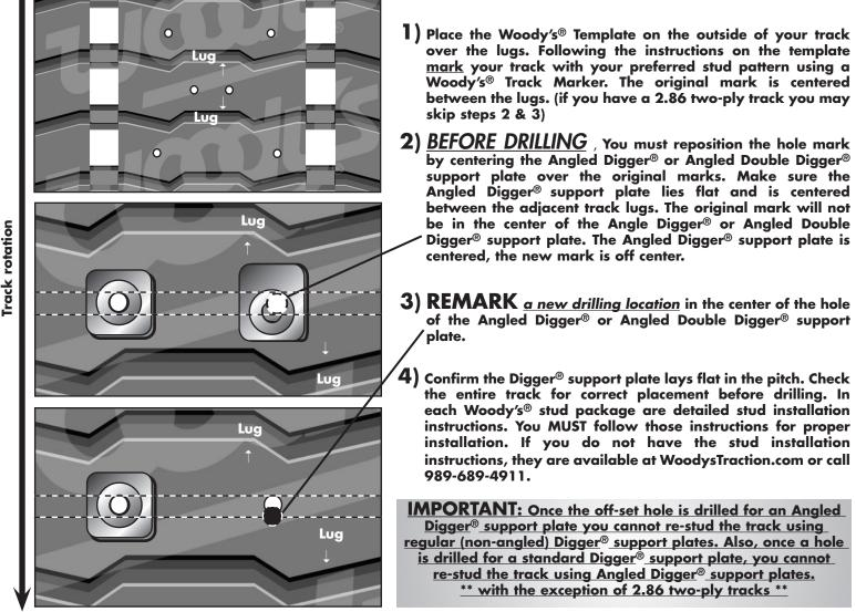
Angled Digger<sup>®</sup> and Angled Double Digger<sup>®</sup> Support Plates require special hole placement, installing them or interchanging them with other support plates may prohibit proper installation.
